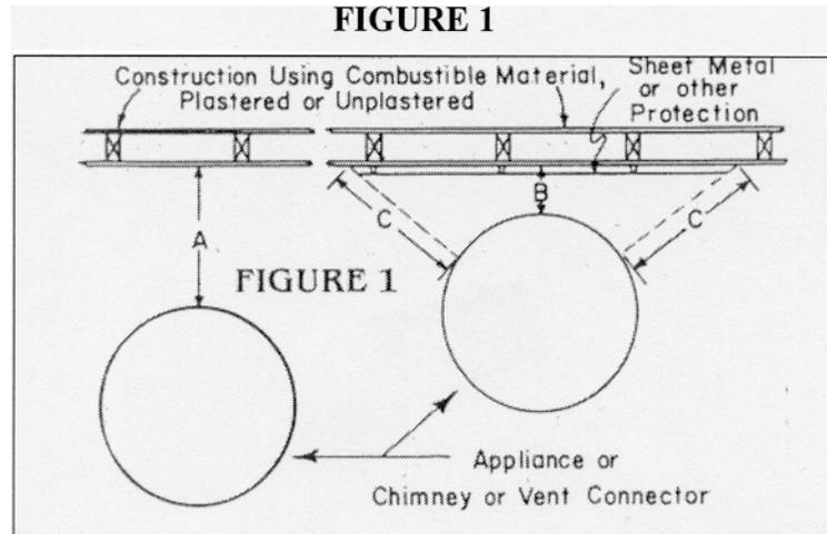
"B" equals the reduced clearance permitted in accordance with Table 2. The protection, applied to the construction using combustible material, should extend far enough in each direction to make "C" equal to "A".
