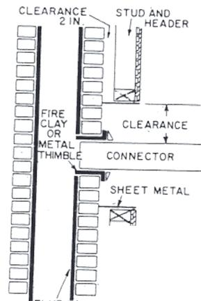
Try to avoid passing a connector pipe through an interior wall. If this must be done, use a ventilating thimble (See Figure 4). The thimble diameter must be at least 12 inches larger than that of the stovepipe, thus giving at least 6 inches of metal-lined, ventilated clearance. If you do not use a thimble, the clearance must be three times the pipe diameter. A 6 inch pipe would need a 42 inch diameter hole cut through a combustible wall.
